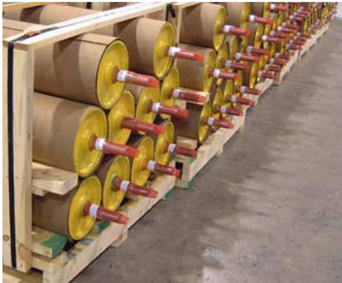
TYPE B: Detachable tapered bushing
